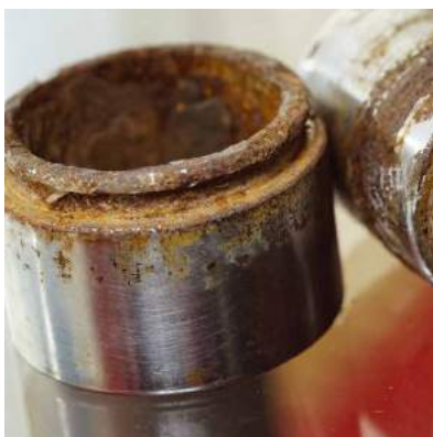
Piston and guide pins corrosion and wedging:
