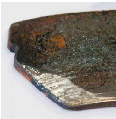
Misalignment, uneven brake pad wear:
