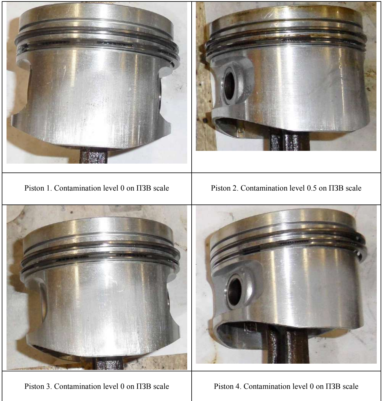
Fig. 44. High-temperature sediments (HTS) after long-term tests (100 running hours) on Lukoil Lux oil added with RESURS NEXT
