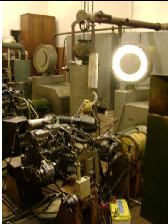
Fig. 2. VAZ-2112 engine on the test bed
