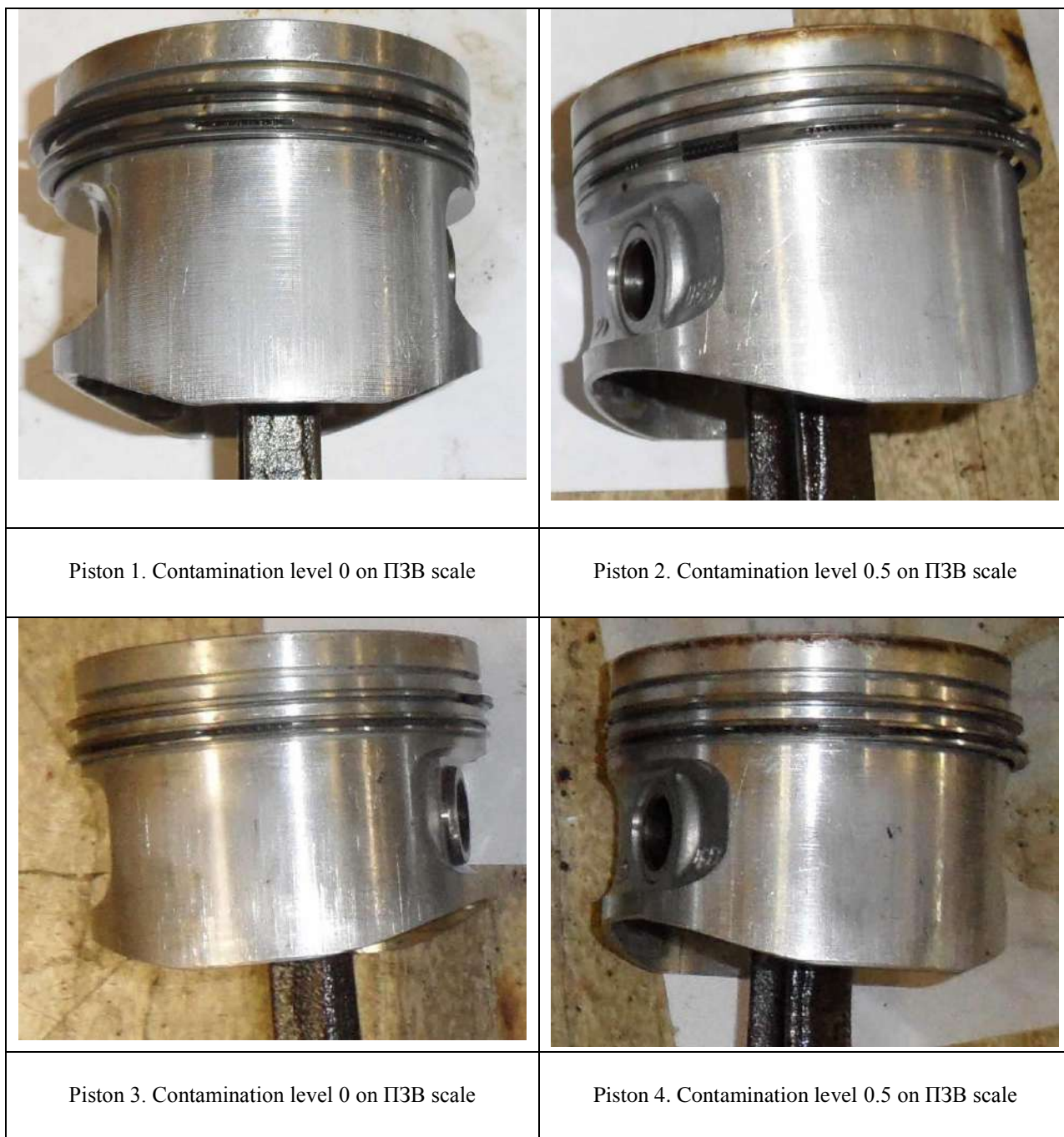
Fig. 45. High-temperature sediments (HTS) after long-term tests (50 running hours, assessment of the duration of treatment aftereffect) on Lukoil Lux oil added with RESURS NEXT
